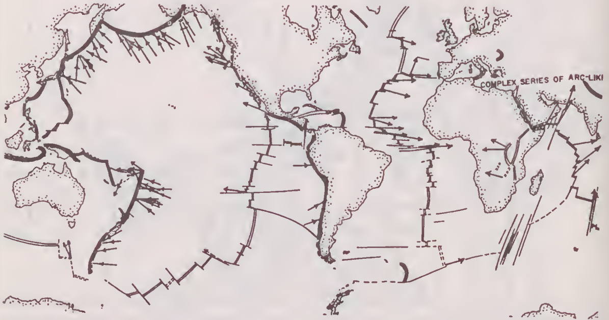
FIG. 5a—Australia, situated well away from the active tectonic plate borders, experiences mild tectonics. The double lines mark the mid-ocean ridges, where new material is added to the plate margins, while the single cross lines represent major transform faults. The thick lines are trenches where one lithospheric plate slides under another, often associated with ocean deeps. Arrows indicate the direction plates are moving with respect to one another. After Oliver, Sykes and Isaacs 1969.
